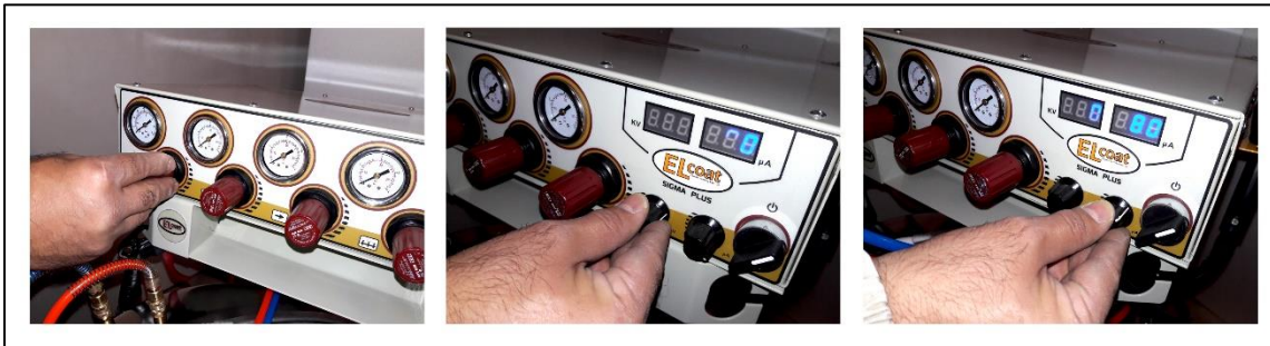
Photo 12. Adjusting the amount of spraying, flow and voltage
