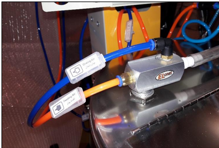
Photo 5. Injector Pump and hoses connections
