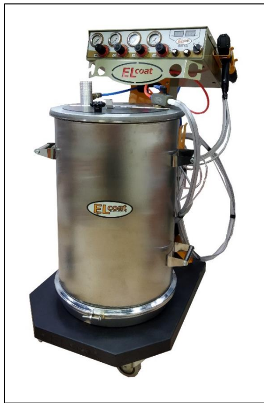
Photo 1. Sigma Plus Powder Coating Machine
