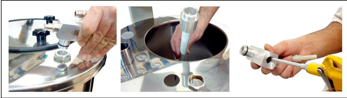
Photo 14. Cleaning the Powder Injector
