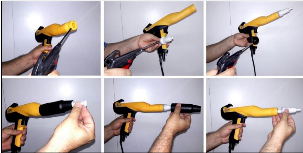
Photo 15. Cleaning the Spray Gun
